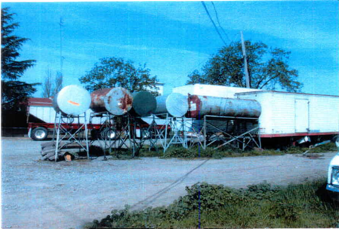
Photograph No. 3. View of center of Mistler property looking west towards six ASTs. According to the property owner AST's are no longer used. Most of them use to contain either diesel or gasoline fuel.
